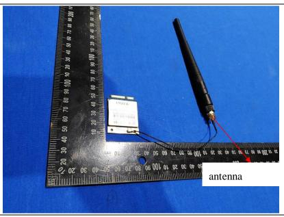
The antenna is a Rod antenna. The best case gain of the Antenna Gain: 3.2dBi;
