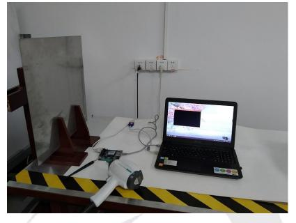
Radio-frequency Continuous radiated disturbance Test 80MHz-1000MHz
