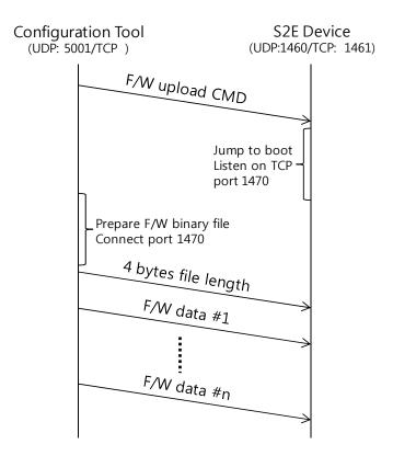
Fig. 9 Firmware uploading timing sequence diagram
