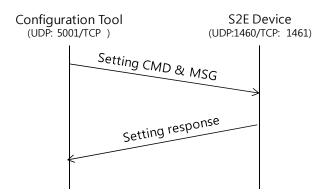
Fig. 6 Setting message exchange timing sequence diagram
