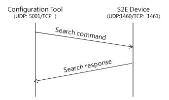
Fig. 3 Searching message exchange timing sequence diagram
