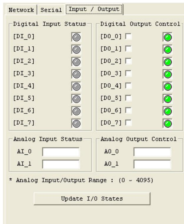
Figure 11. Input / Output Tab of the Configuration Tool
