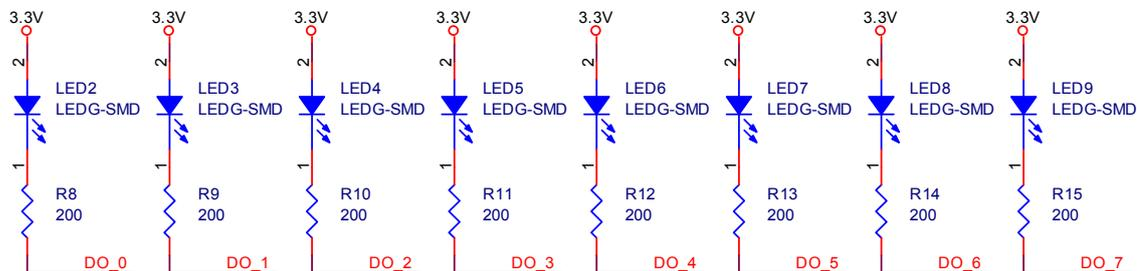
Figure 4. LED circuit of WIZ220IO Base Board
