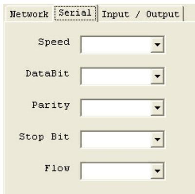
The image shows a screenshot of the 'Serial' tab in a configuration tool. At the top, there are three tabs: 'Network', 'Serial' (which is selected and highlighted), and 'Input / Output'. Below the tabs, there are five rows of configuration options, each with a label and a dropdown menu:
