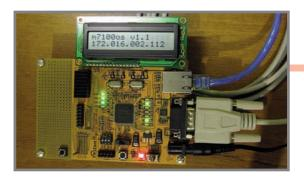
"The m7100os is a network operating system for the WIZnet W7100 iMCU. It consists of a full operating system with a full RTOS with an unlimited number of tasks, priorities preemption, and a reentrant interface for the TCP/IP stack. The W7100 was designed to ease development. It uses a very well-known 8051 core and a hardwired TCP/IP stack. The m7100os just takes advantage of the existing hardware to provide an easier platform for development."—Naubert Aparicio
