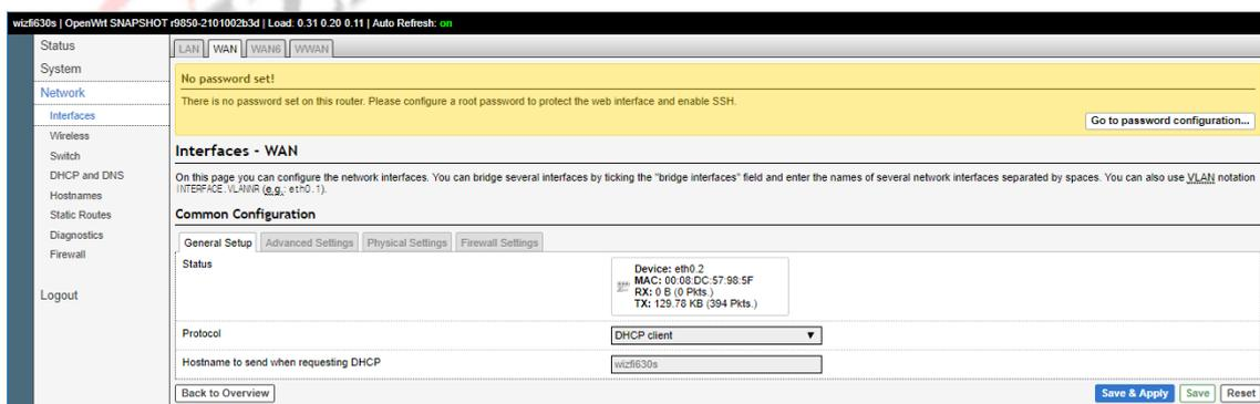
If the Existing network does not support DHCP Server or if you want to use defined IP address, set "Protocol" to "Static address" and enter the IP information of the Existing network as below.
