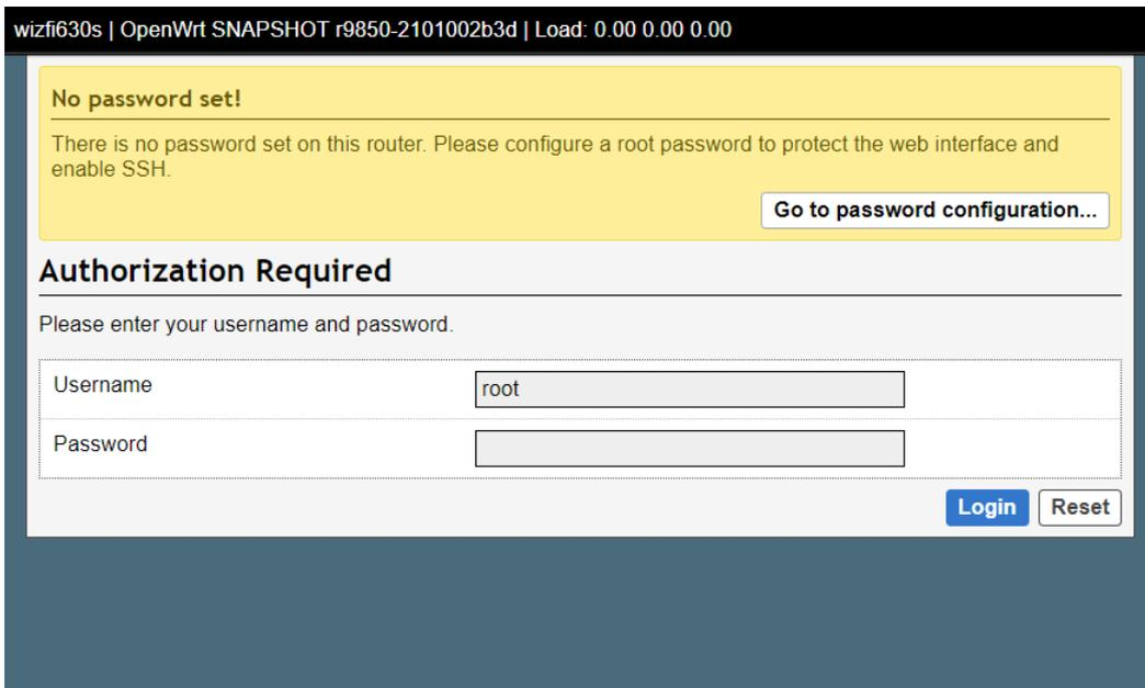
The password is not set by default. Click Login without password to go to the setting screen, or click "Go to password configuration..." to set the password.
