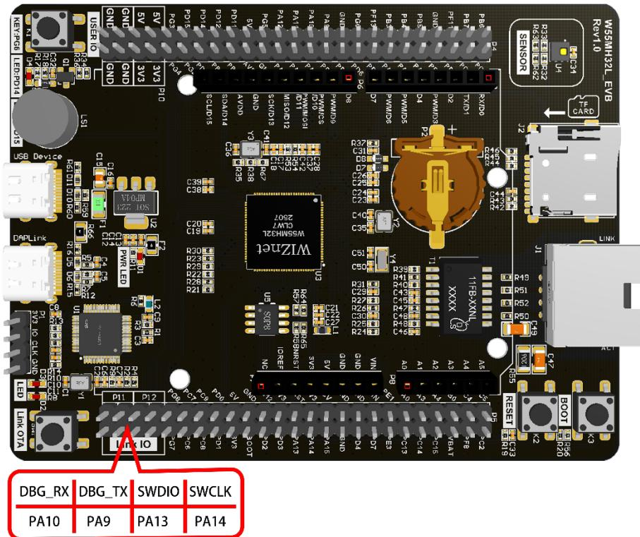
Figure 19 W55MH32 Jumper Cap Connection to WIZ-Link
