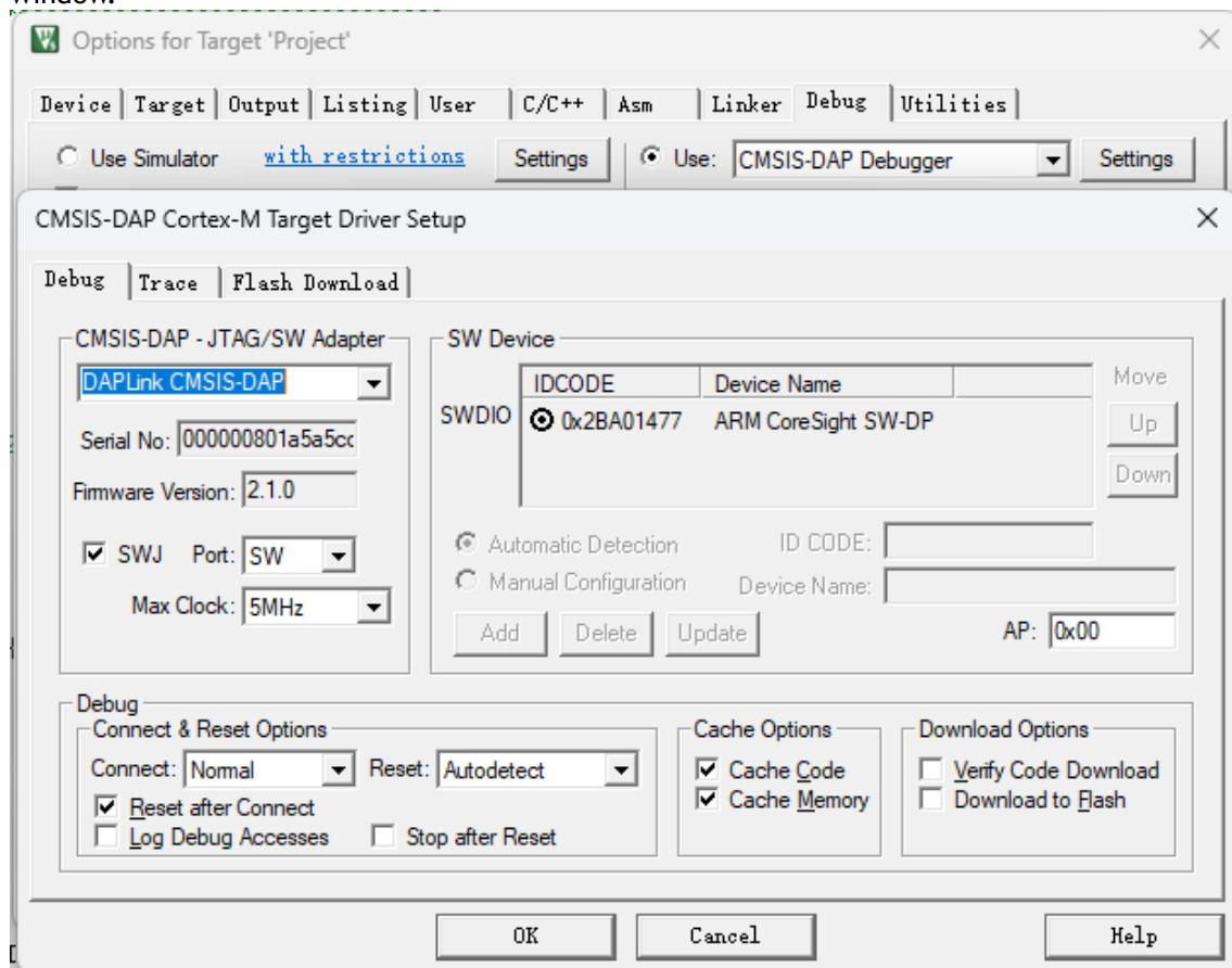
Figure 18 CMSIS-DAP Debugger Configuration
