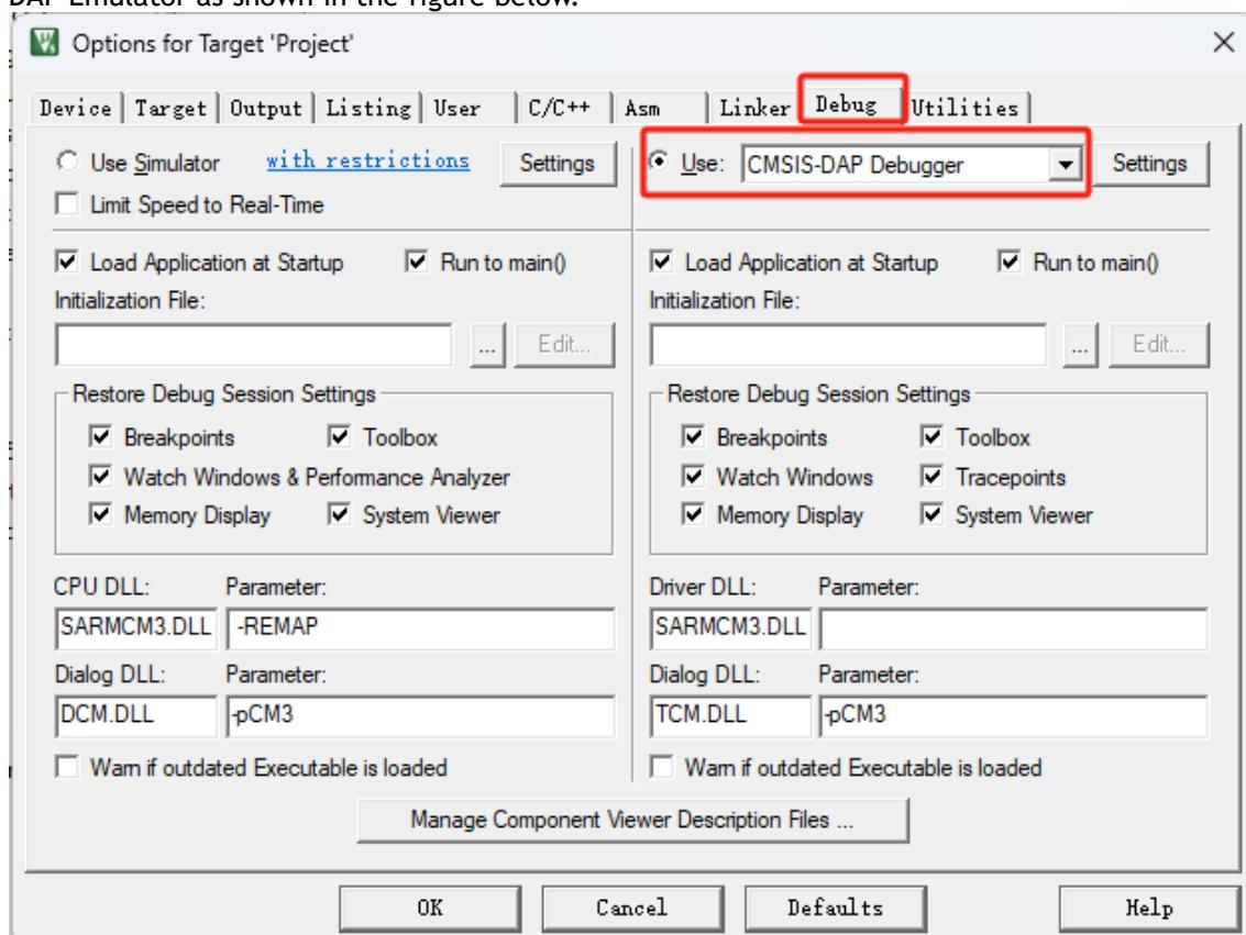
Figure 17 Debug Option Configuration
